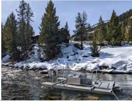
10 - Rotary screw trap on Johnson Creek, ID, installed on March 2, 2022
