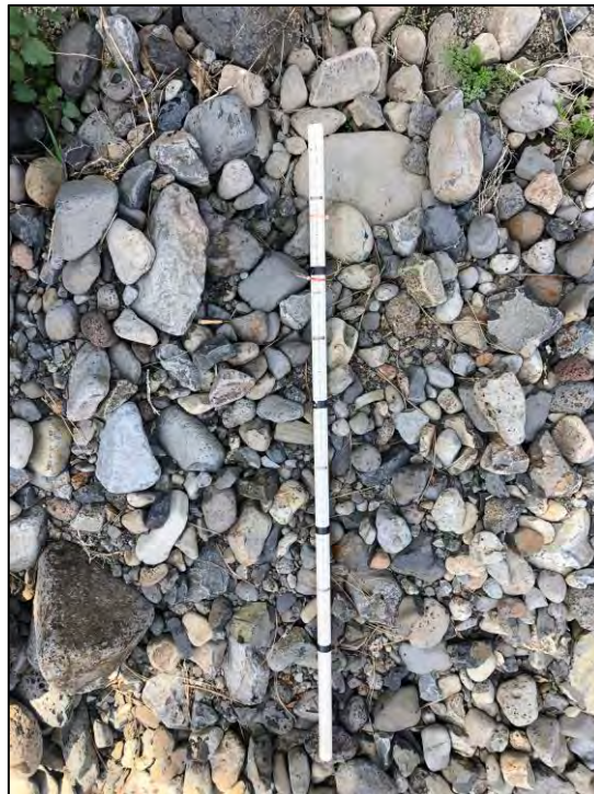
Photograph 10. Existing mobile sediment gradation. Photograph taken downstream of project reach.
