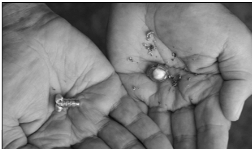
Copper ammo upon impact on the left, lead ammo on the right
